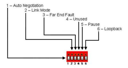
NOTE: All switch changes take effect immediately and will result in a link reset on both ports.
