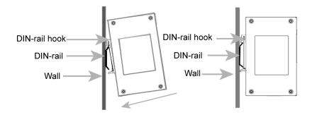
Note: To remove the IDS-105G switch from the DIN-rail, push down slightly on the IDS-105G while pulling the bottom out.
