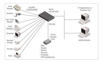
Centralized control and management of multiple deployments is maintained through Perle's Device Manager software resulting in maximum uptime for your remote equipment.
