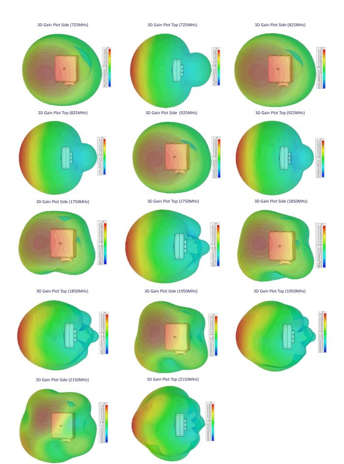
\*3D Patterns show realised gain both elements fed modelled in CST Microwave Studio without additional cable.
